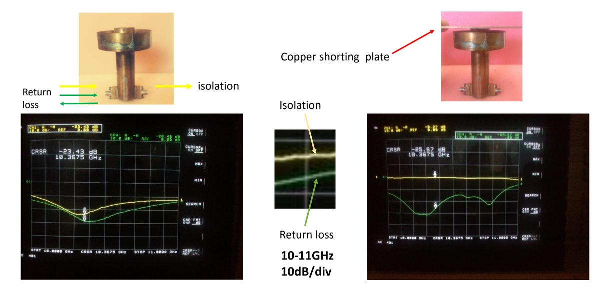
Feed open, with choke at -3.5mm
